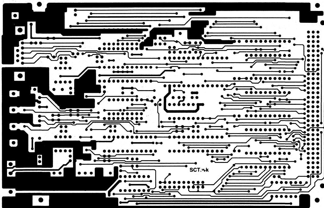
Figure 24. PCB Component Side Layout for Figure 23
